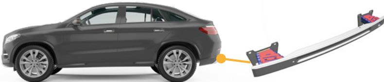
**Lower Rear Bumper:** It is a coloured aesthetical part. Many times, it is difficult to attain the appropriate colour and gloss using post-consumer recycled materials and, at the same time, keep mechanical and physical properties. *REVOLUTION* project will optimise the use of PCR PP, aiming to achieve a 20% weight reduction.
